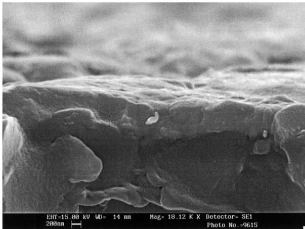
Fig. 5. SEM micrographs of a cross-section of a Ta<sub>2</sub>O<sub>5</sub> film on alumina substrate (from 2 vol.% of metal organic precursor solution).
