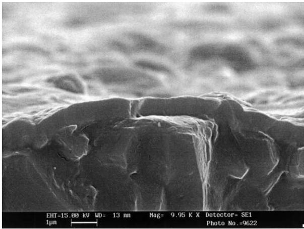
Fig. 4. SEM micrographs of a cross-section of a Ta<sub>2</sub>O<sub>5</sub> film on alumina substrate (from 1 vol.% of metal organic precursor solution).
