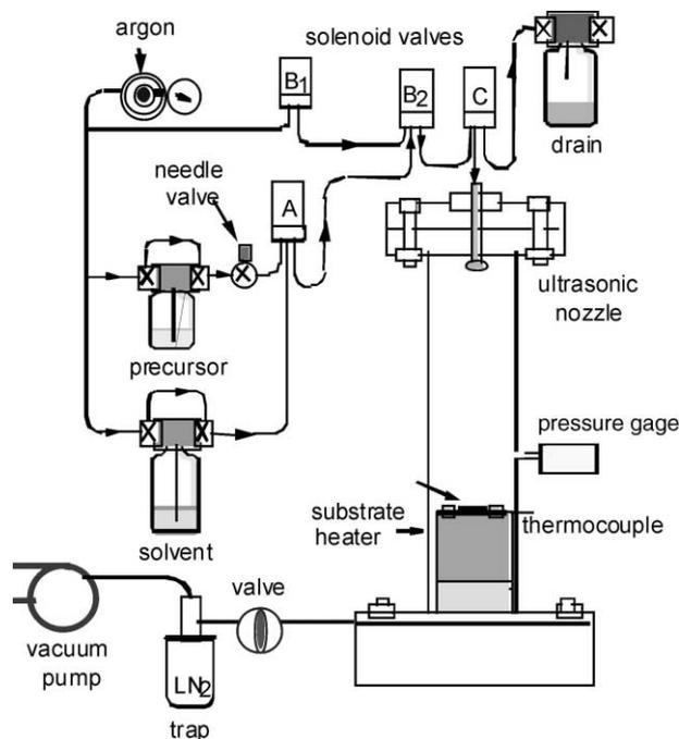
Fig. 1. Schematic drawing of Pulsed-MOCVD equipment with vertical cold-wall apparatus and 5 cm susceptor diameter.
