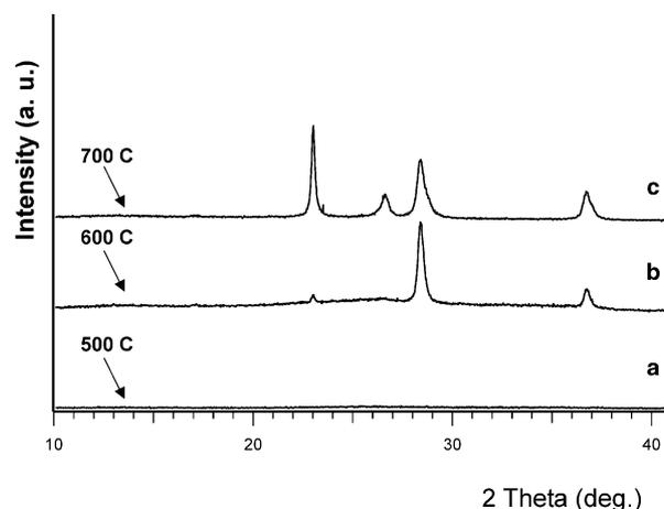
Fig. 3. XRD pattern of the film deposited on Ni substrates. Below 600 °C the films have an amorphous-like structure. For temperatures higher than 600 °C the crystalline orthorhombic  $\beta\text{-Ta}_2\text{O}_5$  phase starts to form.
